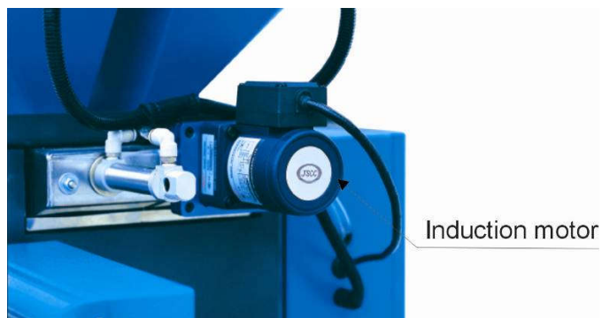
Picture 2-4: Induction Motor Driven Feeding Device
